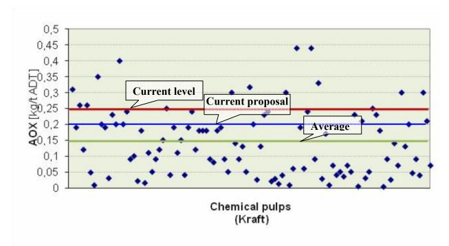
The average AOX value for Kraft pulps of the data in the background report is 0,148 kg/ADT. However, this data does not include CTMP and Recycled pulps which are as followed:
