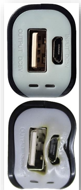
Picture: ICRT/ Which?. The left side shows the USB port of a power bank before the test. On the right side, one can see that the USB port is melted after the test.
